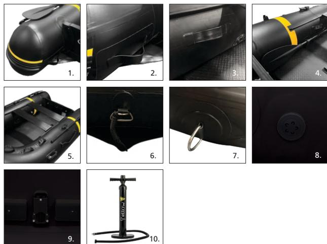
1. The angled stern tubes and the trim flaps at the transom provide a greater planing surface and buoyancy. In addition, the rounded stern tubes with continuous rubbing strakes are less prone to damage.
