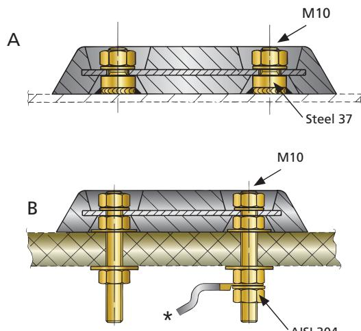
\* Copper wire to connect parts to be protected.
