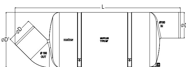
**Note:** Both types should be installed exclusively in combination with an approved reinforced rubber exhaust hose (see pages 130 and 131).
